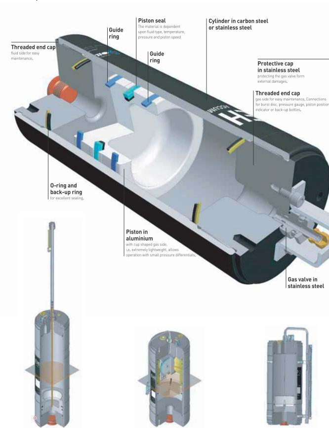
**Piston position indicator.** The piston position indicator is an additional function to the main function of the accumulator, indicating the position of the piston inside the accumulator, thereby ensuring a perfect accumulator operation. The piston position indicator is available with a visual indicator or with electrical monitoring providing 4-20 mA output signal, providing stand-by power during power failure.
